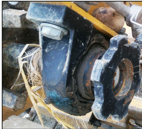
Tone wheel attached to the weighing belt drive shaft.
