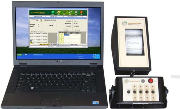
*Figure C-1: Front view of HM-800 components*
