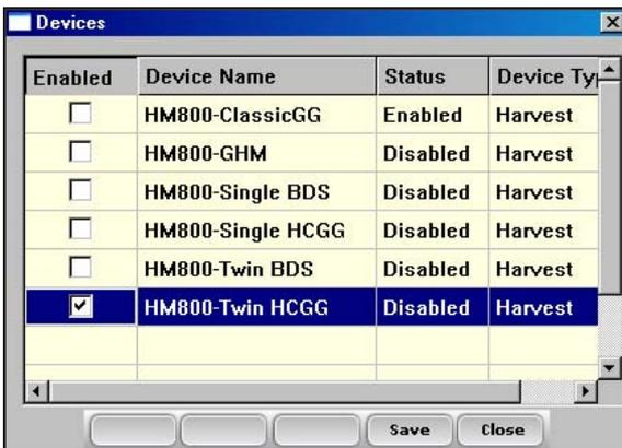
**Figure 2-3: Devices screen showing the HM800-Twin HCGG as enabled**
