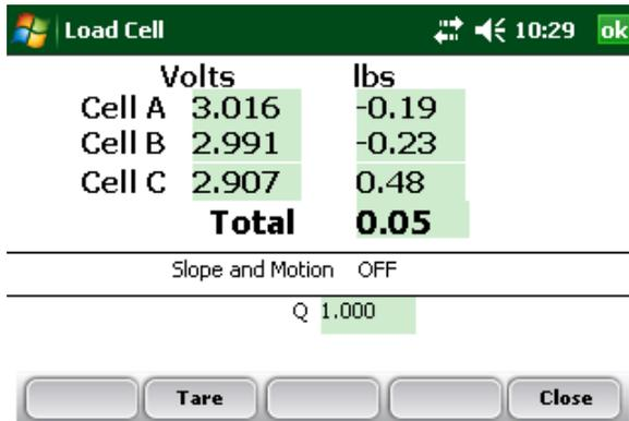
*Figure 4-2: Diagnostics Load Cell screen*
