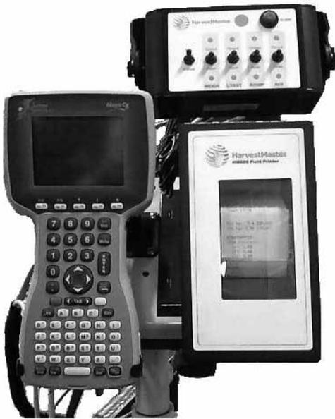
*Figure C-1: Front view of HM-800 components*
