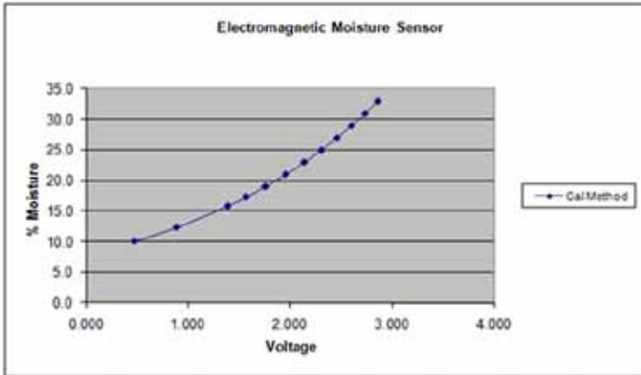
*Figure 3-17: EM Sensor moisture curve*
