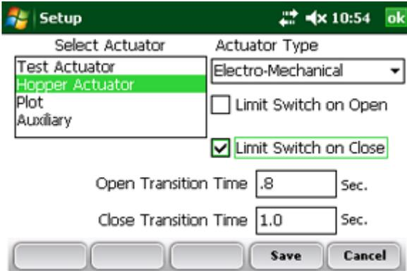
**Figure 3-24: Actuator Setup screen**
