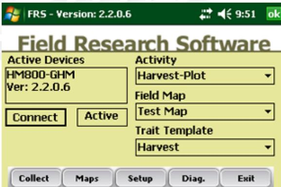
*Figure 5-1: The Generic Harvest Module appears in the Active Devices box*
