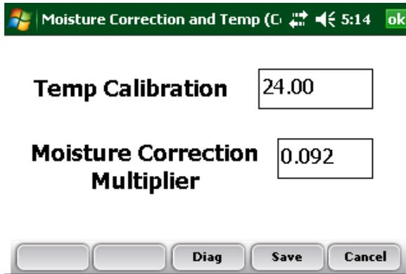
*Figure 3-16: Temp compensation screen.*
