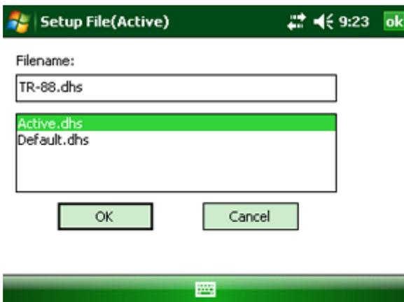
**Figure 3-26: Naming a new setup file**
