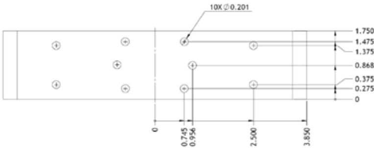
The next two diagrams are for mounting the printer.
