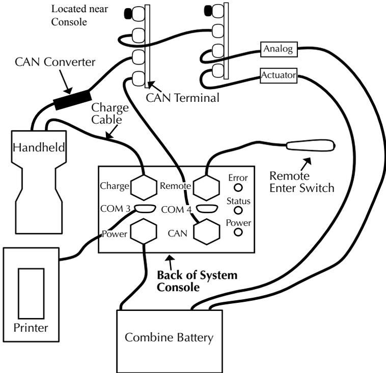
**Figure C-2: Cable connections for the HM-800**
