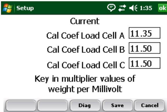
**Figure 3-6: Edit Weight Calibration screen**
