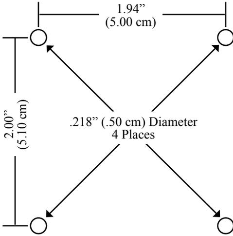
Below is pictured the system console mounting diagram.
