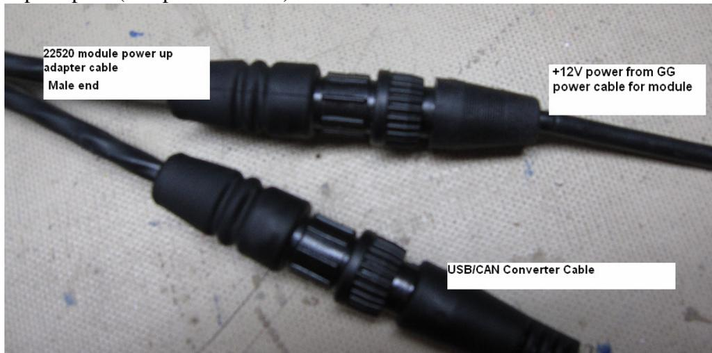
12. Plug the power plug and CAN plug of the other end of the power up adapter into the module to be recovered, press the power button on the system console if programming a system console and make sure the module powers up. The other modules should turn on with the use of the module power up adapter. (See Picture Below)
