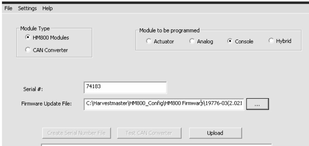
9. Make sure power is supplied to the modules power cable.
