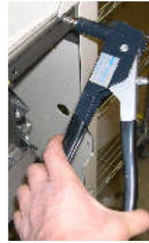
6. Check to make sure the button snap socket is secure.
