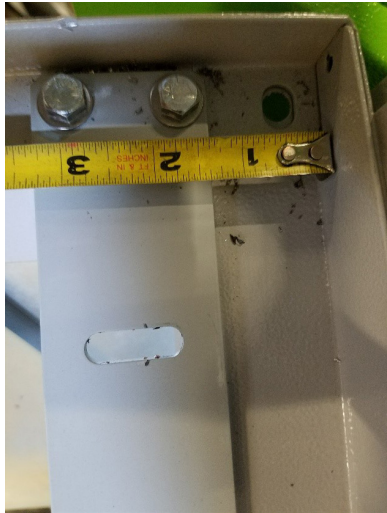
Place inside support bar 1-3/8" from edge
