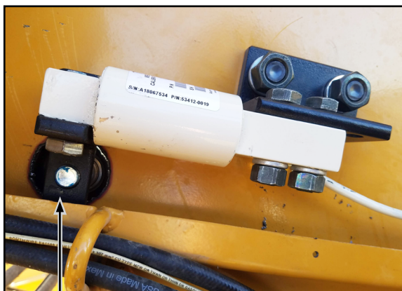
Idler wheel axle hex bolt in the load cell idler mount
