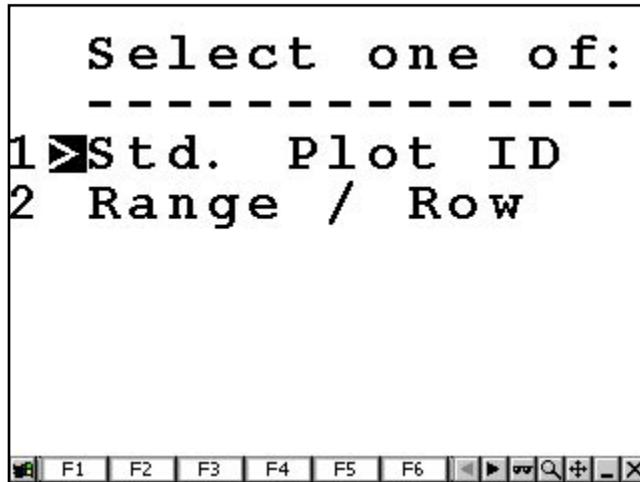
4) Select the areas that you need to change. Press *Enter* or down on the round arrow key move to the next option. The field map is generated by pressing *Enter* or the down arrow on the round key after you select the desired Type setting.
