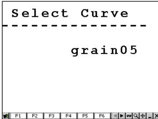
3) Select the percent or volts you are changing, and enter your new sample moisture percent or moisture volts. Press *Esc* to save your changes to the moisture curve and advance to the Cal TempC (Calibration TemperatureC) screen.
