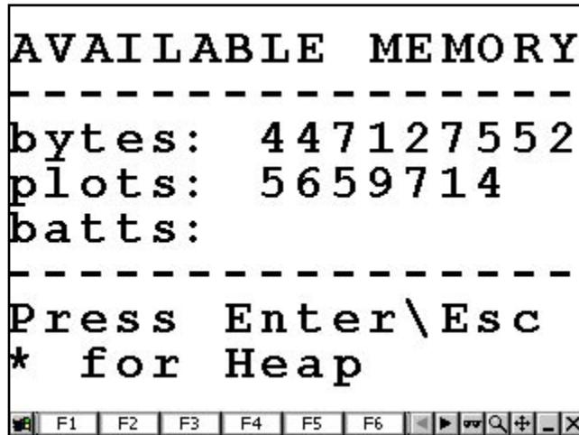
The Available Memory screen gives you the information for bytes, plots, and batts (battery). You can press \* to replace the bytes reading with the Heap reading.
