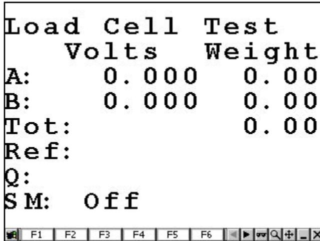
Note: Typically, the user would place a known weight in the bucket to test the weight calibration.
