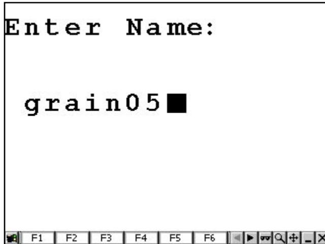
*Note: We recommend using a name that is similar to the type of grain that the moisture calibration curve is being calculated for; such as CORN, WHEAT, or WET-CORN. We recommend adding the year to the end of the curve name (i.e. CORN01).*
