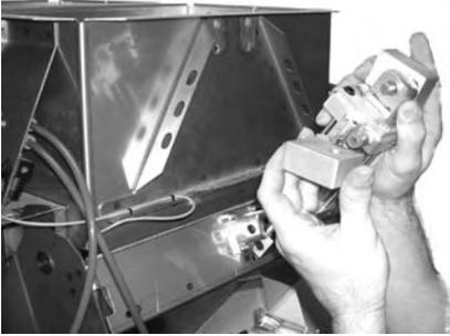
***Figure 9-9: Slide the cylinder off the clevis rod***
