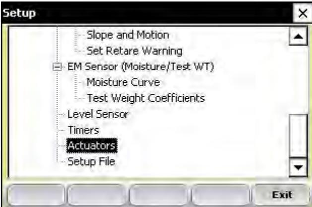
**Figure 3-34:** Double-tap **Actuators** from the **Setup** menu to access the **Actuator Setup** screen
