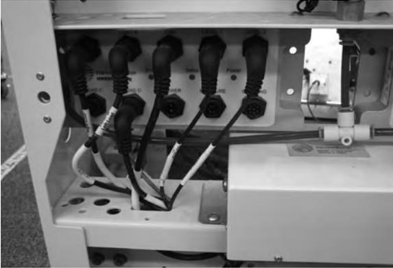
*Figure D-11: Cables under cross beam and attached to analog module*
