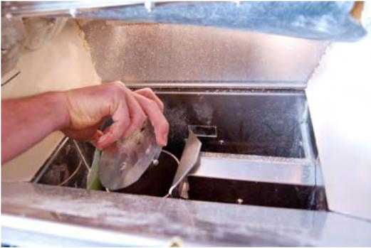
**Figure 4-15: Weight being placed in BDS cup**
