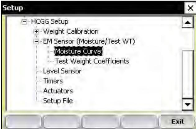
***Figure 3-17: Setup screen with Moisture Curve screen selected***
