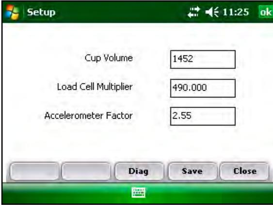
Figure 4-13: Test Weight Setup Screen
