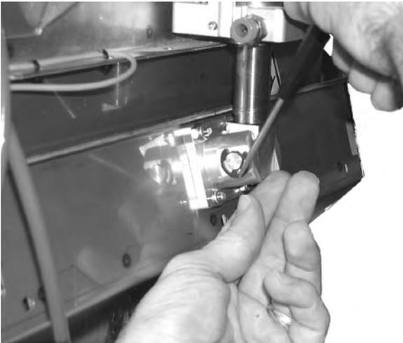
***Figure 9-6: Removing the e-ring from the pin***
