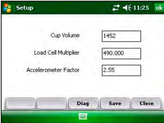
*Figure 4-17: Test Weight Setup Screen*
