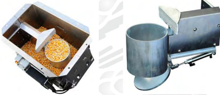
**Figure 4-1: BDS cup inside bucket and outside of bucket**
