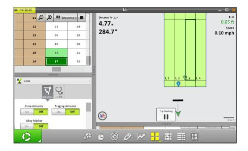
**Step 4**: Proceed through the plots at a consistent speed. Mirus triggers the planter automatically.
