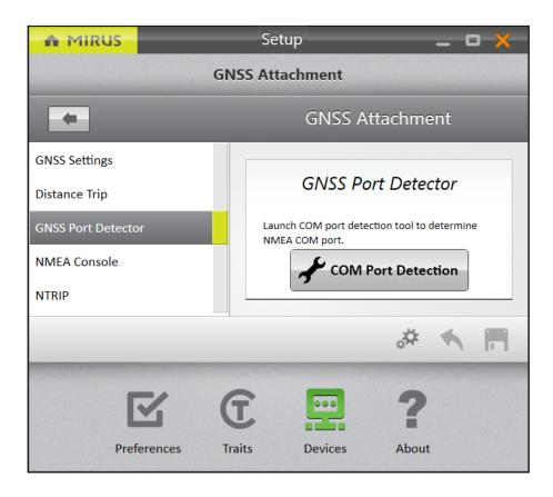
Mirus opens the GNSS Port Detection box and detects the ports.
