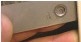
5. Make sure the button snap socket is flush with the surface, as shown in the picture on the left. Squeeze the tool and pop the rivet.
