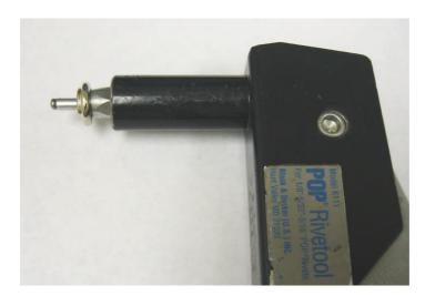
3. Insert the end of the pop rivet into one of the seven holes shown on the next page.
